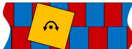
Figure 22: Linear measurement setup - Rotation of iC-MU Series about its own axis
