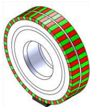
Figure 3: Radial magnetic pole wheel example
