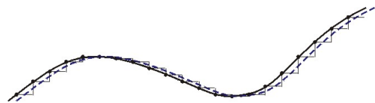
Figure 3.7: Time delay due to DA-conversion
